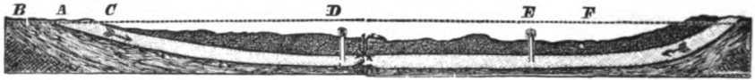
FIG. 3.—Section showing certain conditions governing artesian wells. A, a porous stratum; B, C, impervious beds below and above A, acting as confining strata; F, height of water level in porous bed A, or, in other words, height of reservoir or fountain head; D, E, flowing wells springing from the porous water-filled bed A. (After Chamberlin.)
